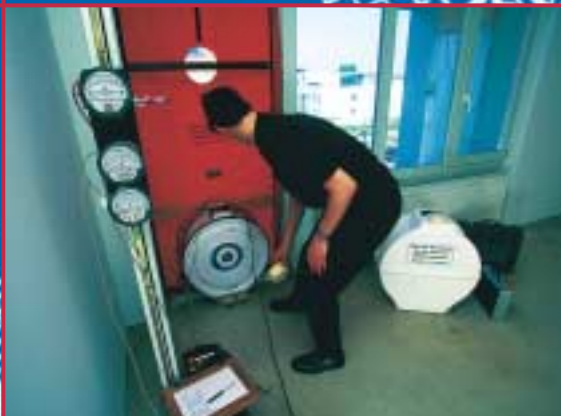
THE BLOWER DOOR TEST SHOWS UP GAPS
