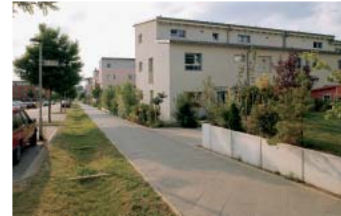
MULDEN-RIGOLE ROADSIDE DRAINAGE HOLLOWES
